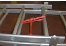
Use a load strap with cam buckle (maximum load at least 500lbs) to join the top rung of the mobile ladder to the 3rd rung from the bottom of the mobile ladder. This way you'll be able to put the ladder vertically without it collapsing.
