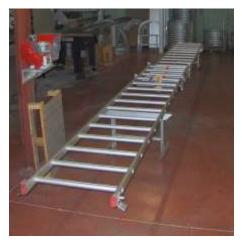
Clamp the two ladder sections together by clamping two coinciding rungs in between 2 wood boards with a C-clamp.
