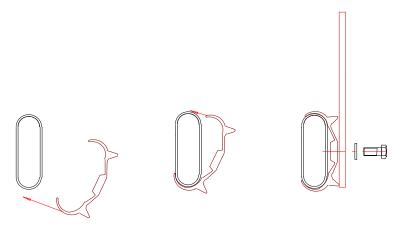
If this bracket is meant to withstand vertical loads, it needs to be secured to the ladder beam by a blind rivet, as shown below.
