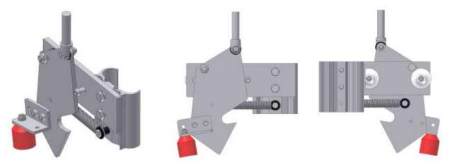
The latch can be opened from the bottom with a push rod, as showed in the picture below. At the same time another rod is mounted alongside the ladder up to the top where it can be pushed down in order to open the ladder.
