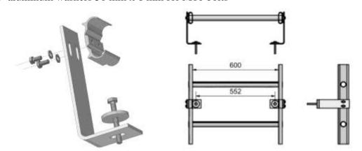
The ladder fixing anchors have to be drilled 552 mm (21 3/4 in) apart. Each anchor bolt is fitted into an oblong hole in the ladder fixation base that allows for a 20 mm (0.8") clearance.
